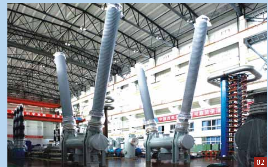
01: Commissioning of 800kV Dead Tank Circuit Breaker 02: 800kV Dead Tank Circuit Breaker in test
